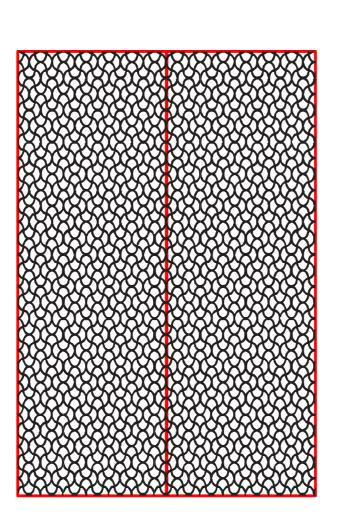
PETG - Do one piece then wait 5 minutes. Seperate pieces when lasering and watchout for buckling of material
