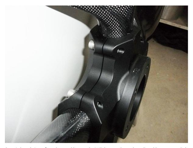
One pitch angle is confirmed we could proceed... BUT then we changed to adjustable, so we needed a new hub design. This were CNC machined Aluminium. (image)
