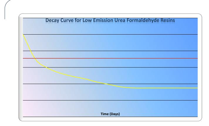
Source: Decay curve : Orica Adhesives, Back ground level : testing undertaken at Plywood House, Brisbane Australia, February 2004 (0.009 ppm)
