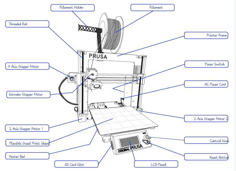
**COMPONENTS** LCD Panel AC Power Cord Z Axis Stepper Motor 2 **Control Knob Reset Button** Flexible Steel Print Sheet Z Axis Stepper Motor 1 **Extruder Stepper Motor** Filament X Axis Stepper Motor SD Card Slot Threaded Rod Heater Bed **Filament Holder Printer Frame** Power Switch
