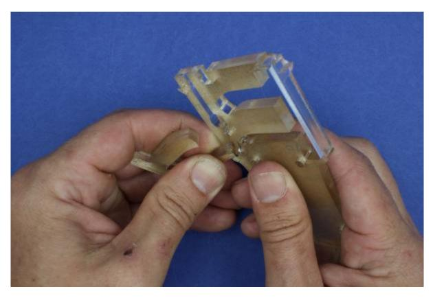
And peel off the plastic cover on the LED panel
