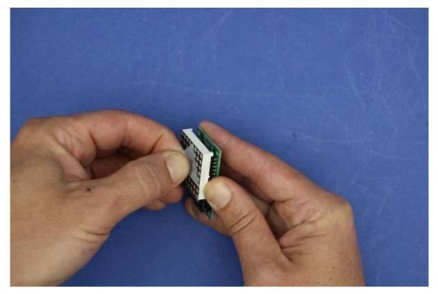
Then take the LED panel off its board. You can use the back of the pliers
