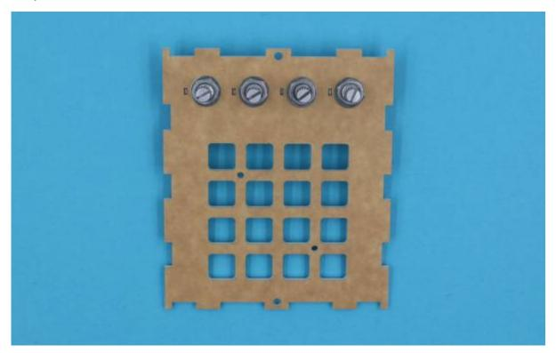
Insert the Trellis keypad with the rubber keys from the back. Make sure your trellis wires are at the bottom (opposite the pots) and that the text on the Trellis board is correctly oriented, the Adafruit logo should be on the bottom right.
