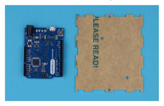
Align the Leonardo and the base with the bolt holes. Insert the bolts from the bottom of the base. The additional power port will be in the way for one of the nuts, simply angle the bolt and screw on the nut. It is possible to remove the power port as we don't use it.
