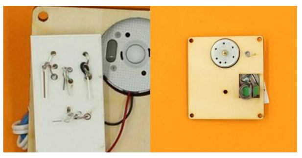
Make sure that none of the twisted wires are touching another lot of twisted wires, and test your circuit by giving the cog on the motor a sharp spin (anticlockwise).
