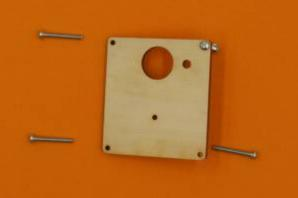
Thread a nut onto each screw as you insert it, and this will prevent things from falling out when you move the plate.
