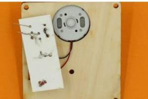
As you can see, the motor fits into the round hole, and the toroid will fit into the rectangular hole when everything is in place.
