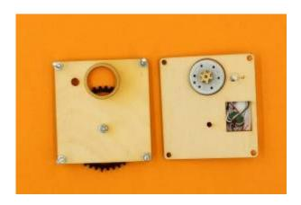
Turn the top plate upside down, and mount the middle plate onto the corner screws, making sure the small cog engages with the large cog.
