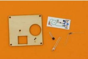
Take up the LED, and you should see that one leg is longer than the other. LEDs only work when electricity flows through them in the right direction, and the different legs help you to insert the LED correctly (the long leg is the positive terminal).
