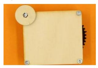
You may need to press down firmly on the bottom plate to attach nuts to the corner screws (pressure also helps keep the motor support in place).
