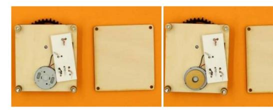
Without dislodging the motor supports, guide the bottom plate onto the corner screws.
