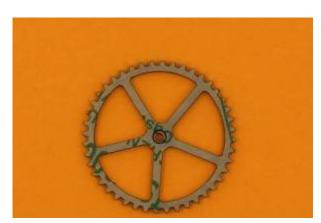
Now you can push out the spacer, and peel the protective paper from all the bits.
