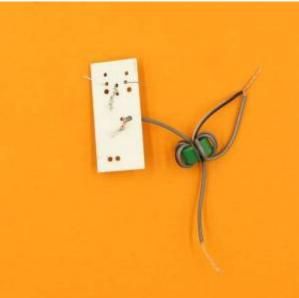
The <u>striped</u> single wire from the toroid follows the **solid green** line, and pushes through next to a transistor leg.
