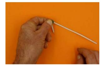
Now take the long end of the wire, while keeping hold of the toroid with your other hand, and loop the wire back through the centre of the toroid.
