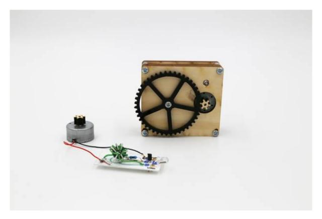
This is a small manually powered gear-driven generator made from ply and acrylic, with a Joule thief circuit.
