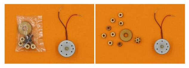
Push the wooden cog firmly on to the motor shaft (it has to be a tight fit).
