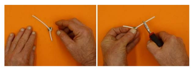
If it has not been done for you, separate the protruding wires (use a knife or cutters, or just pull them apart with your fingers). Do this on both ends.
