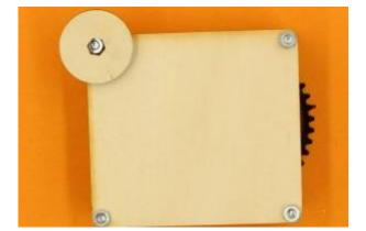
You may need to press down firmly on the bottom plate to attach nuts to the corner screws (pressure also helps keep the motor support in place). Use the wooden spanner to tighten the nuts.
