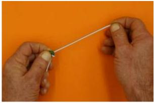
Continue threading the wire through, until there are 4 or 5 loops around the toroid. More loops actually reduces the effectiveness of this device, and it will still work with 4.
