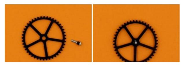
Now insert the screw (with the cog attached) though the smallest hole on the top plate. Thread a nut on from underneath, and tighten with your wooden spanner.
