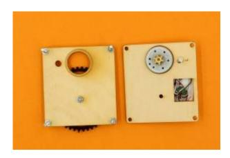
Turn the top plate upside down, and mount the middle plate onto the corner screws, making sure the small cog engages with the large cog.
