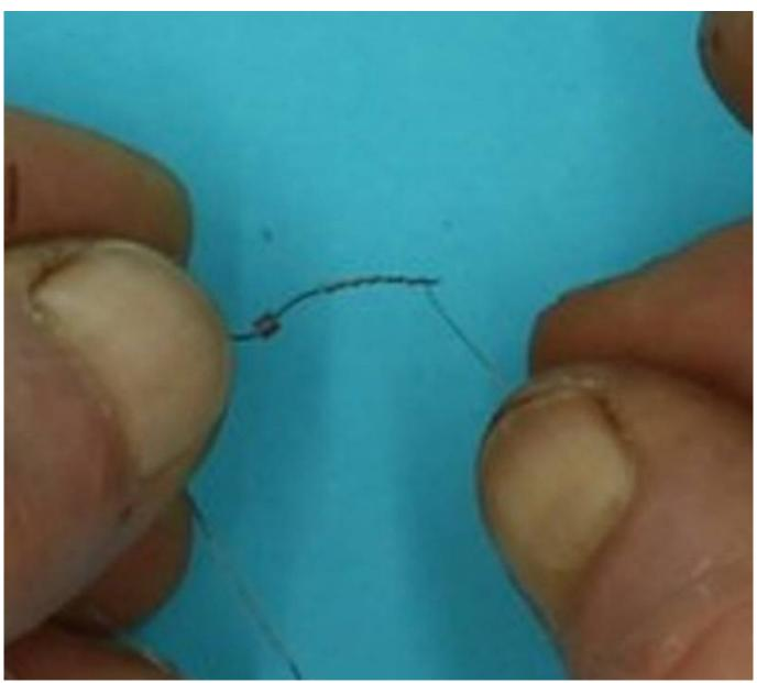
The crimp was slid down over the joined wires, and crushed closed with pliers.
