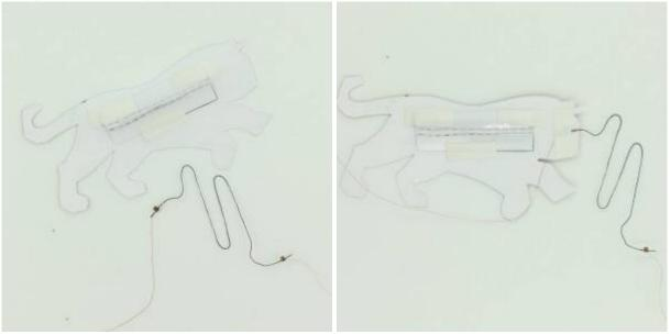
Make sure the memory wire is oriented so that movement will occur in the direction you want - this is why the wire is not straightened at this point - in this case, it will concertina along the same plane as the flat tiger image when activated.
