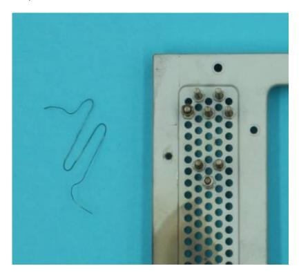
Lead wires had to be attached to either end of the memory wire shape so that the device could be incorporated into the final design. A length of multi-strand core copper woire was stripped, and disassembled to provide the thin copper wire required. Lengths of this wire were then firmly attached to the ends of the memory wire using small (imm) metal crimps available as jewelry making supplies. Firm crimping with pliers was needed to ensure a good connection.
