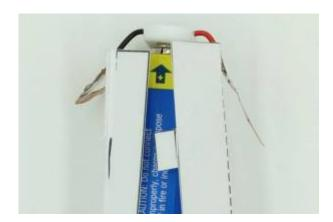
Tape the holder closed (the tab will help hold things in place), and bring the attached wires through the slots provided. Now tape the terminal connections down onto the sides of the holder, making sure that the copper contacts are not covered.
