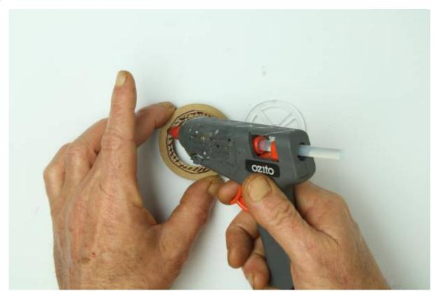
Apply glue to the marked area, and glue the acrylic hub to the cardboard ones, lining up the edges with the marked circle.
