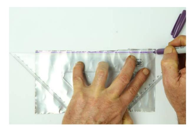
Turn over the sheet, and using a straight edge, mark a line along the long side about 5mm inside the ragged, cut edge.
