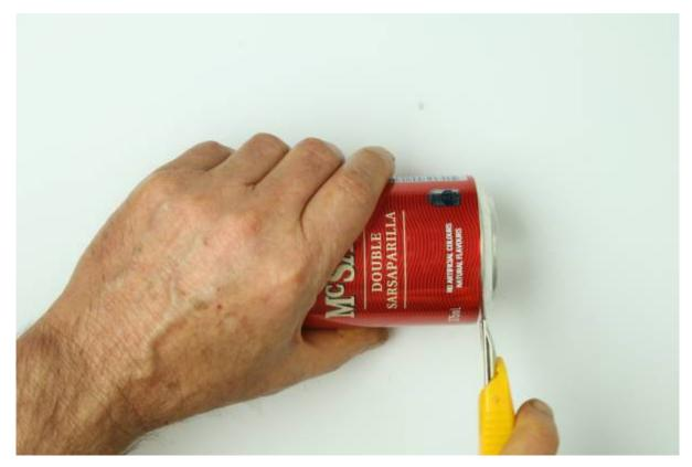
Holding a can firmly with one hand, use a craft knife to slice around the end.
