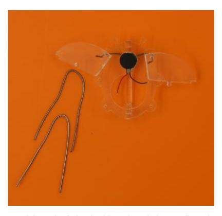
Turn the Vibrobot over and the ends of wire should now be pointing up. Slip a wing over each leg, using the small hole provided.
