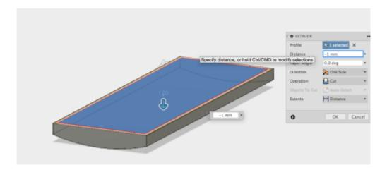
Using the design history, click the sketch for the offset you just created. Then once in delete the offset constraint. You can now move the bottom line up to allow room for a button. click exit Sketch
