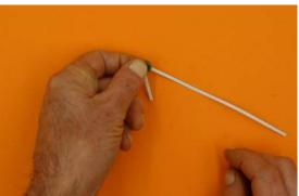
Now take the long end of the wire, while keeping hold of the toroid with your other hand, and loop the wire back through the centre of the toroid. Then, pull the wire tight.
