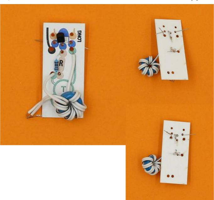
The joined toroid wires go through the hole at the bottom on the diagram, and can hang free until the next step.
