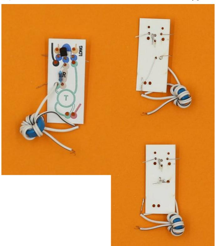
The striped single wire from the toroid follows the solid green line, and pushes through next to a transistor leg. Insert the striped wire, and twist these two together (bend them away so nothing is touching).
