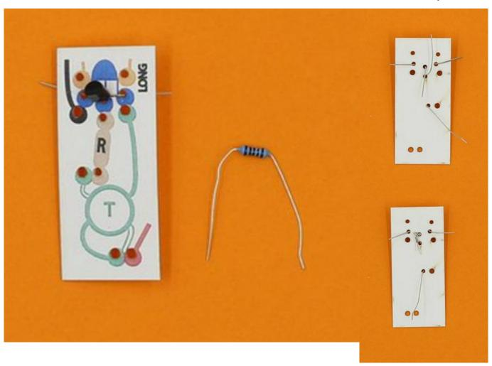
When you look at the back of the circuit board, two wires are now adjacent: the middle one from the transistor and one from the resistor.
