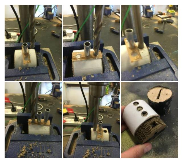
check alignment of holes on example plug are within tolerance
