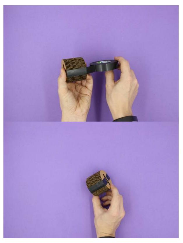
Before we move on, insert your plug into the white tube and make sure the plug spins properly without any or little friction. Feel free to use sandpaper to remove some of the rough parts on the tube. Align the holes of the plug and the tube, you might need to flip the plug 180 degrees for the best result.
