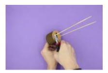
Grab two of your magnets and insert them into the small hole on one of the sides of your plug. Face the magnet front/back outwards. Make sure it is lower or flat with the surface otherwise it may cause unwanted friction when turning the plug. It doesn't matter what direction the polarity is going for the time being. We will match the other magnets with it later.
