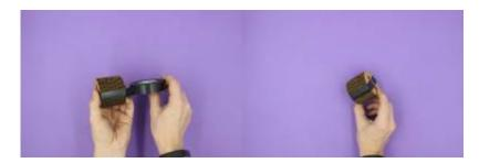
Before we move on, insert your plug into the white tube and make sure the plug spins properly without any or little friction. Feel free to use sandpaper to remove some of the rough parts on the tube. Align the holes of the plug and the tube, you might need to flip the plug 180 degrees for the best result.
