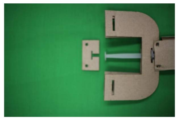
The end piece also comes as upper and lower parts, each with a slot for the plunger flange of the top syringe.
