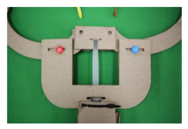
Push the split pins (or paper brads) through the slot in the yoke, and the inner holes in the claw arms.
