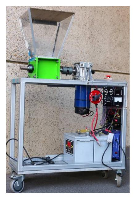
Shredder components were laser cut by external service providers according to the design files available from the https://preciousplastic.com/en/ website, with the following modifcations:
