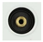
The spur is made of brass and the internal gear is plastic. This means the brass gear grinds the plastic until the arm servo falls off, requiring a replacement shoulder mount.
