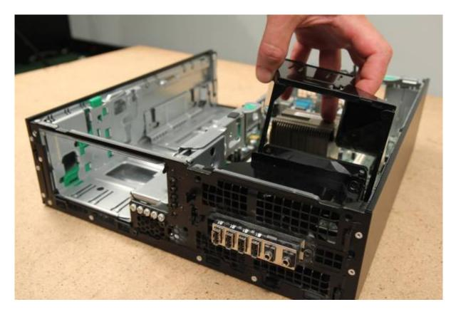
Four tabs on the fan connect it to the chassis. Squeeze in the top two tabs:
