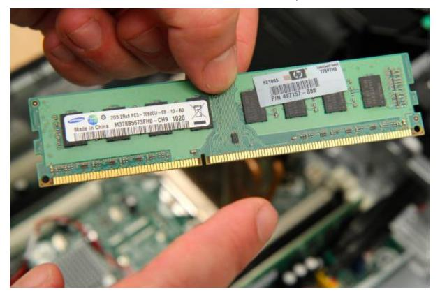
Don't touch the memory chips. Static electrical discharge can easily damage or destroy them.
