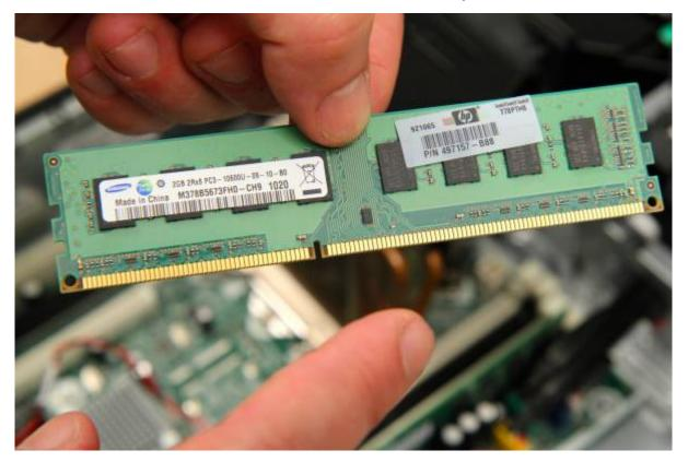
Push in firmly. Tabs on the socket will grab and hold the stick. Repeat with the second RAM stick.
