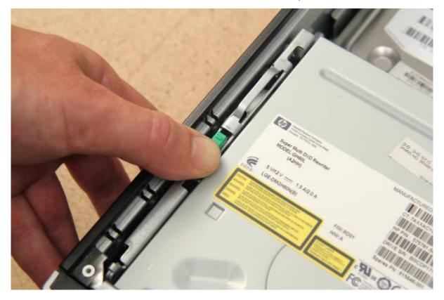
Slide the drive forward, and lift straight up to remove from the bay.
