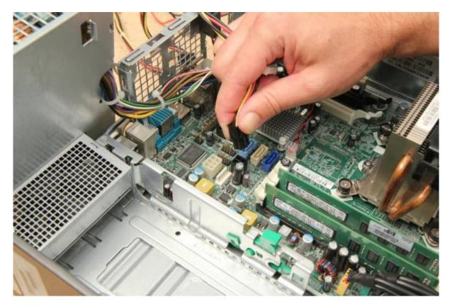
Clear the cables, then tilt the PSU and lift straight out.
