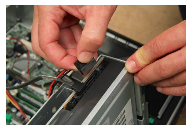
Ensure cables run through the cable clip.
