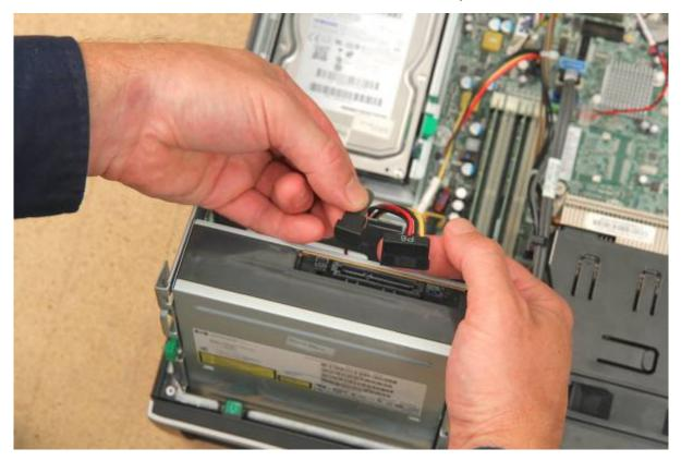
Unclip the cable guide and free the cables.
