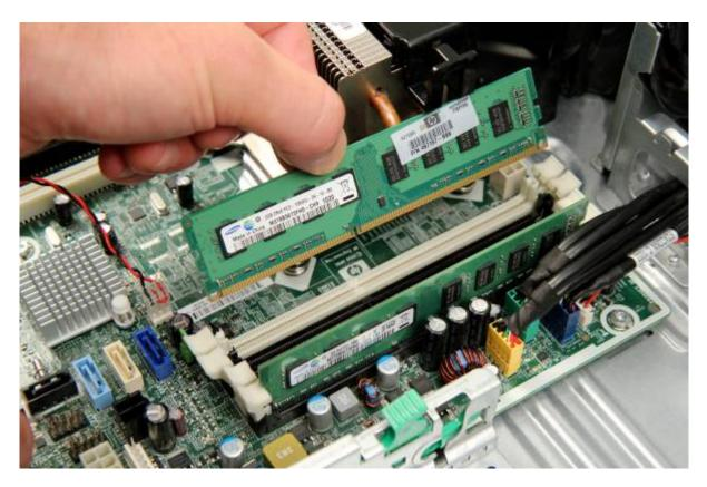
Don't touch the gold parts on RAM, as skin cells/sweat can cause corrosion
