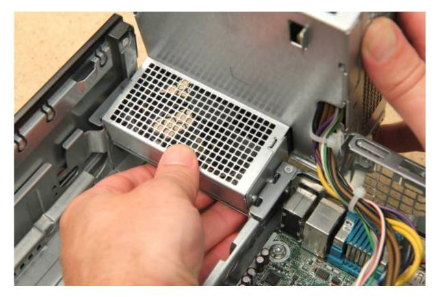
Re-connect the PSU cables to the motherboard (they only fit one way).
