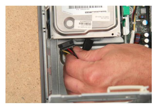
Push down the green tab on the right of the drive bay. Slide the hard drive forward.
