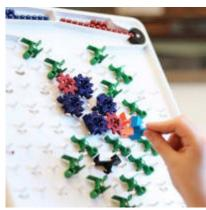
Turing Tumble is a new type of game where players build mechanical computers powered by marbles to solve logic puzzles. Use ramps, crossovers, bits, interceptors, gears, and gear bits to build marble-powered computers that can generate patterns, do logic, count, add, subtract, multiply, divide, and much, much more.
