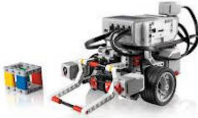
LEGO MindStorms is a platform to support the development of programmable robots based on LEGO building blocks. It contains an intelligent brick computer that controls the system, a set of modular sensors and motors, and LEGO parts from the Technic line to create the mechanical systems.
