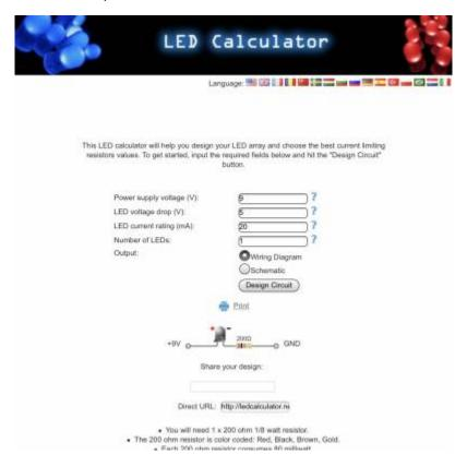
This calculation shows we would need a 200 Ohm 1/8 watt resistor. When shopping for resistors, make sure you get a resistor that is 200 Ohm, the wattage is the minimum required so if you cannnot find a 200 Ohm 1/8 watt resistor, a 200 Ohm 1/2 or 1 watt resistor would be fine.
