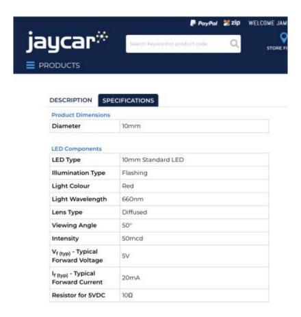
Assuming we are using a 9V battery, we can use the resistor calculator to work out the resistor we need for the circuit.
