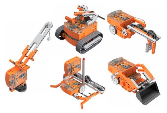
The Edison is an Australian based robot which is LEGO compatible, the Edison can be converted into a myriad types of machines with the EdCreate extension pages, LEGO blocks, or whatever you might have lying around! Edison can be coded via its own block-based coding language - EdBlocks, or via barcodes, and can be driven with any infra-red remote control unit.
